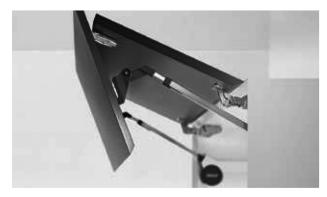
Mechanism designed for heights between 72 cm and 96 cm, based on the **BLUM AVENTOS HF** system, whereby the two-piece front folds in the middle during opening. Easy to open, lockable in any position, soft and quiet close, thanks to the BLUMOTION system. Three-dimensional adjustment of both fronts and stability even with wide fronts. Optional SERVO-DRIVE (see paragraph 3.7). LGA-certified for over 40,000 cycles.
